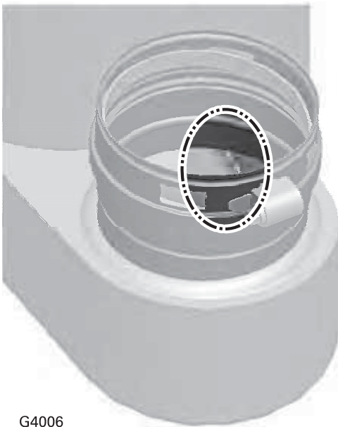
Figure 83 Recuperator flueway drain holes
